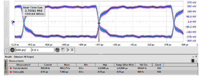
Fig. 24. Measured eye diagram of the divide-by-16 recovered clock at 720MHz.
